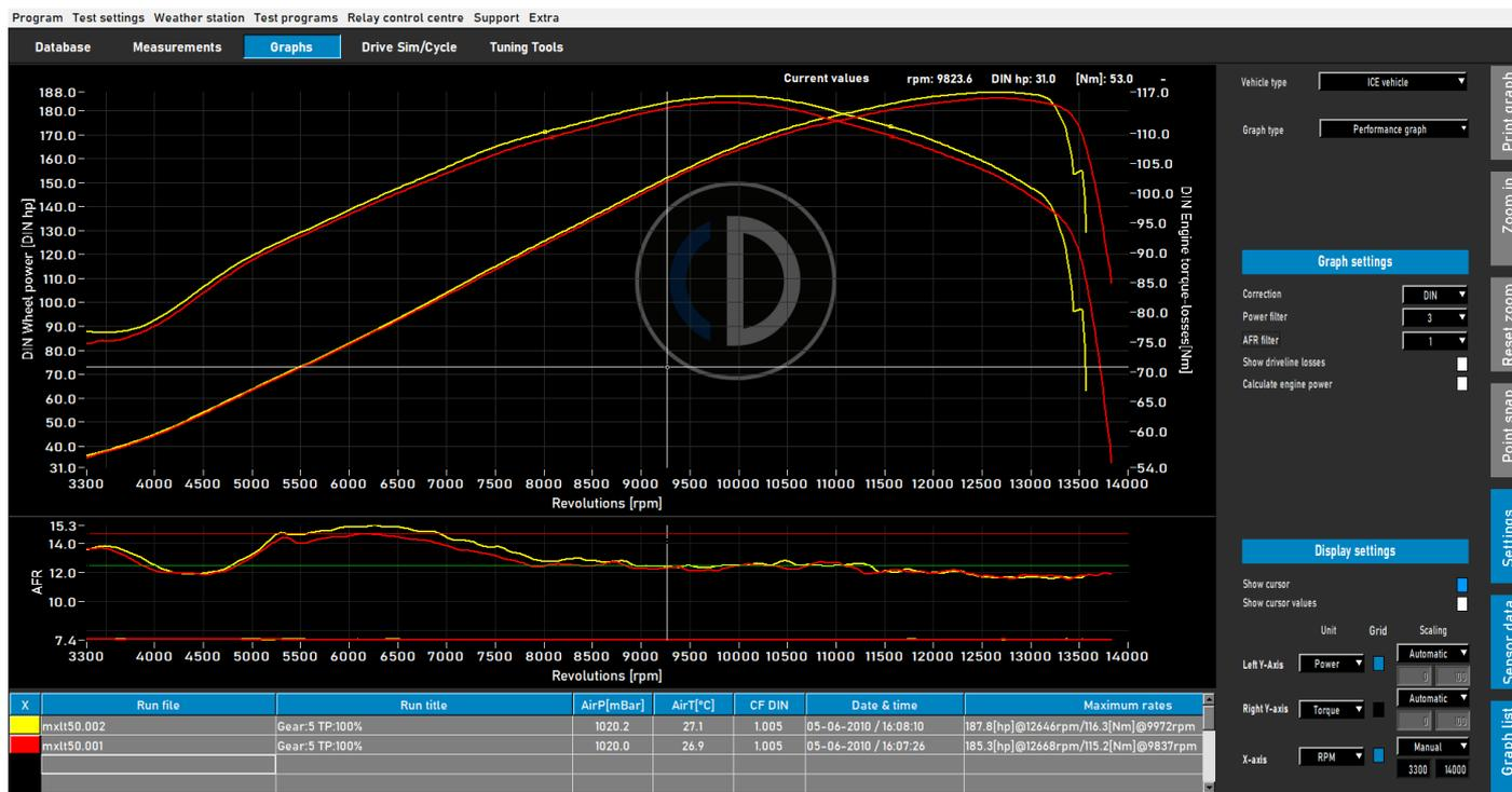
Once a test is made, automatically the graph screen is opened as shown above. The made test is plotted and previous tests or previous selected tests are also visible. It's possible to load different tests from different brands and types from the database to show in the graph screen. Power (left Y-axis) is always displayed, besides torque (right Y-axis) and drive line losses which can be switched on and off by double clicking on the graph area. The X-axis can be either RPM, speed or time.
