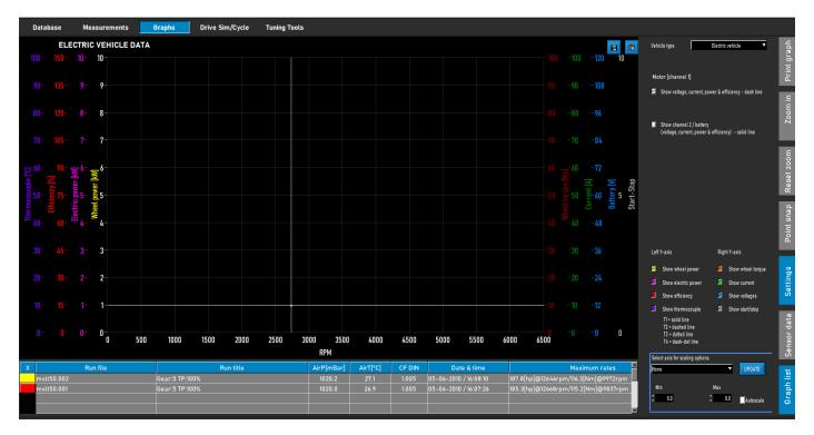
*GRAPH SETTINGS, Correction factor;* select the required correction factor, DIN, SAE or EEC/EWG. Weather station data is always recorded, changing before or after is therefore always possible. It's advised to always use a correction factor for correct data comparison.
