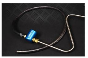
can cause a delay because the exhaust gas has to travel through the tube before it reaches the sensor. When using this method make sure the tube is inserted far enough into the exhaust.
