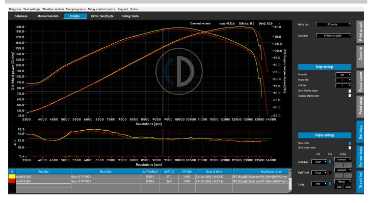
Once a test is made, automatically the graph screen is opened as shown above. The made test is plotted and previous tests or previous selected tests are also visible. It's possible to load different tests from different brands and types from the database to show in the graph screen. Power (left Y-axis) is always displayed, besides torque (right Y-axis) and drive line losses which can be switched on and off by double clicking on the graph area. The X-axis can be either RPM, speed or time.
