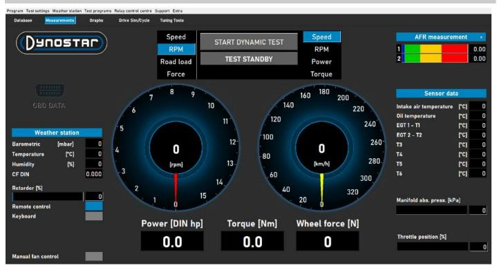
The *Measurements* screen, is the main operation screen. In this screen all live data are displayed and tests are performed. The center of the screen is formed by the two large gauges. These gauges can show the engine RPM, vehicle speed, power, torque, road load and force.
