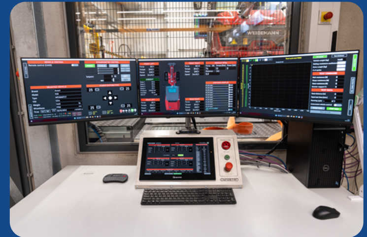
Control panel with emergency stop, reset, buzzer and HMI with 15.6" touchscreen
